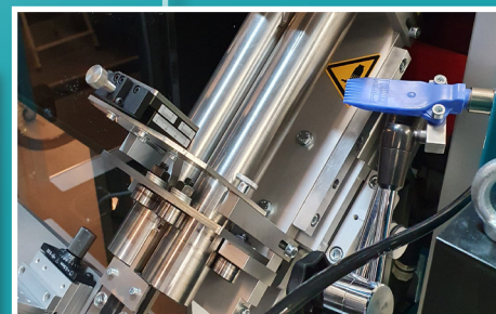
Stabilization of the products with spinning rollers
